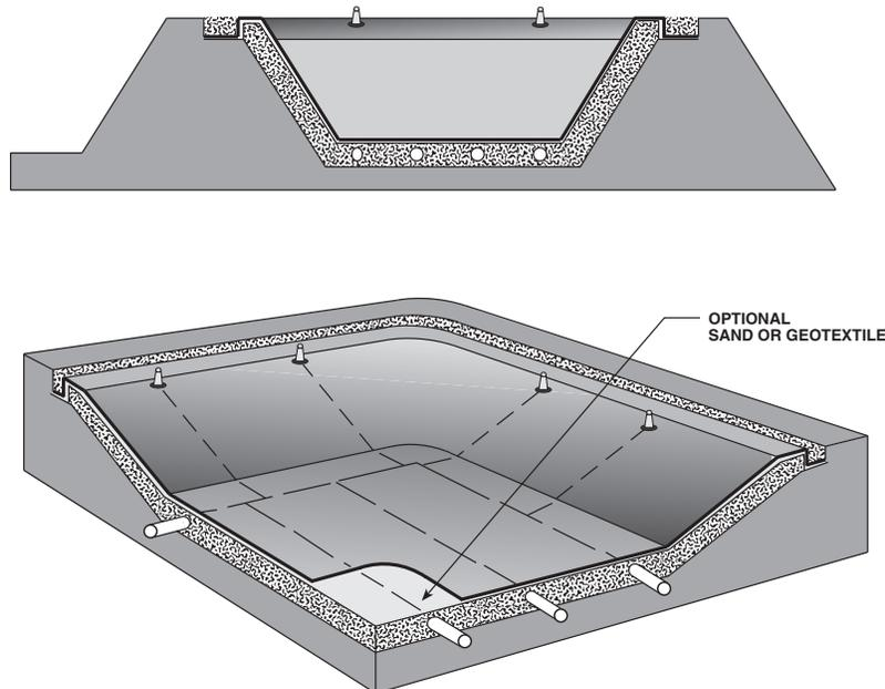
**Figure 4. Gas drainage - Pipes, or pipes/geosynthetic layer**
