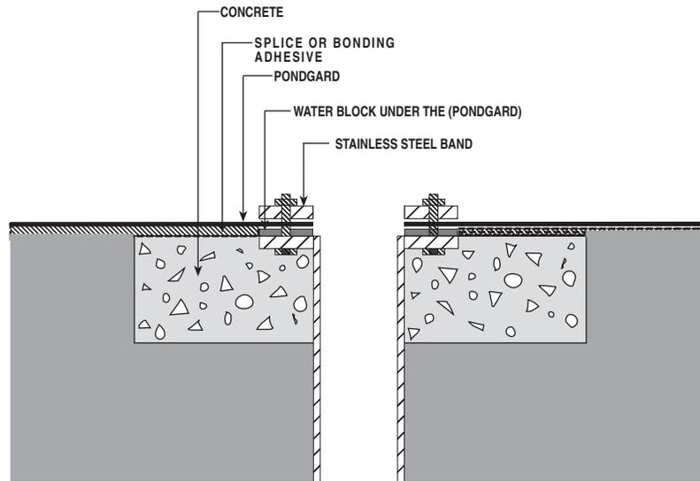
**Figure 13. Water discharge with steel flange collar**
