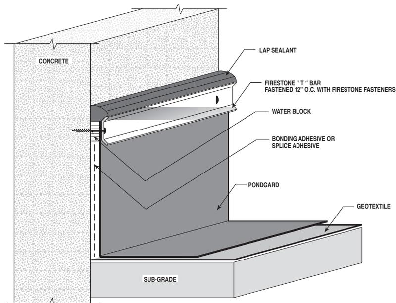
Figure 10. Connections to concrete (above the waterline)
