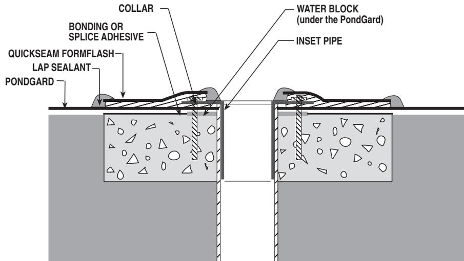
**Figure 14. Water discharge with inset pipe**
