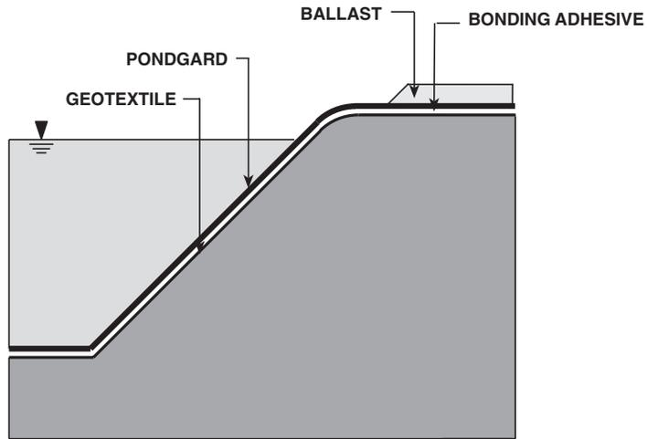
Figure 5. Top of slope ballast
