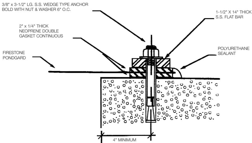
**Figure 10. Connections to concrete (below the waterline)**
