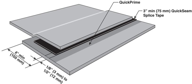
Figure 15 EPDM seam
